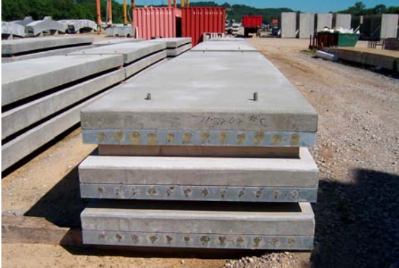
Fig. 8 Maysville Waterfront (Precast/Prestressed Concrete Slabs) Photo provided by Carr Concrete (A subsidiary of R.W. Sidley, Inc.)
