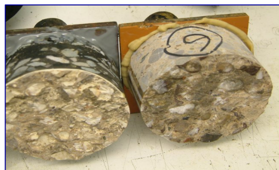
A38 (M) Test results showing failure mechanism in asphalt or concrete substrate
