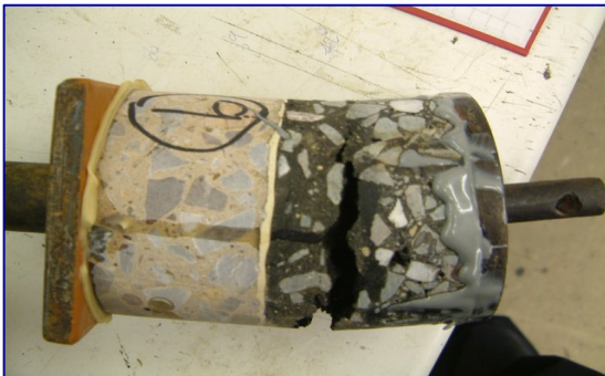
A38 (M) Test results showing failure mechanism in asphalt or concrete substrate
