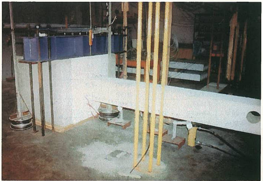
Fig. 4. Encased pile test setup.
