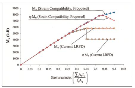
Fig. 4. Proposed strain compatibility design moment for section in Answer A4, versus current AASHTO-LRFD solution.
