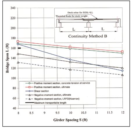
Fig. 1. NU1100 span capacities, System B.
