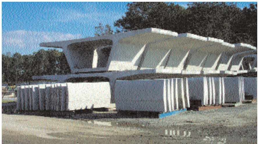
Fig. 12. The fast pace of the schedule required the precaster to turn over 30 forms daily to maintain production. Parapets and segments shown here were stored at the plant site. Photo courtesy: Bayshore Concrete Products.
