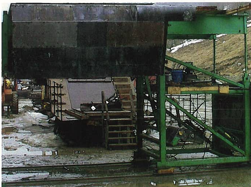
Fig. 5. Mandrel or core form.
