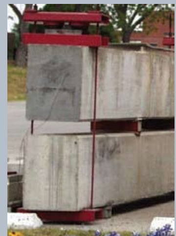
Figure 5. Shown are the beam-specimen details and test setup for the beam corrosion test series. Note: 1 in. = 25.4 mm; 1 ft = 0.3048 m.
