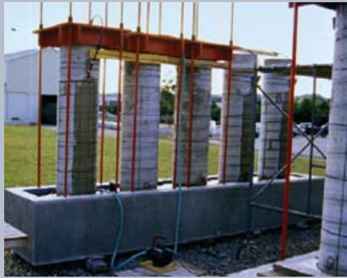
Figure 8. Shown are the test setup and column-specimen details for the column corrosion test series. Note: 1 in. = 25.4 mm; no. 6 = 19M.
