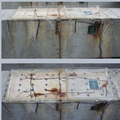
Figure 7. Shown is a beam corrosion test series example of specimen condition prior to internal examination and generalized corrosion ratings for phase I internal examination beams. Note: 1 ft = 0.3048 m.
