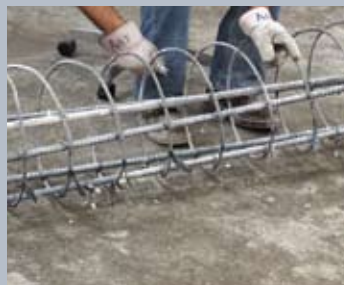
Figure 10. Shown is the column concrete removal and dismantling of reinforcement for the column corrosion test series.
