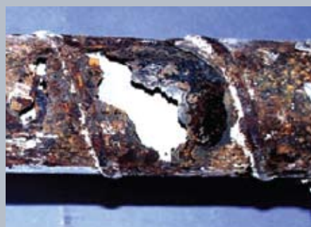
Figure 16. Pictured are bleed-water voids and duct corrosion from the beam corrosion test series.
