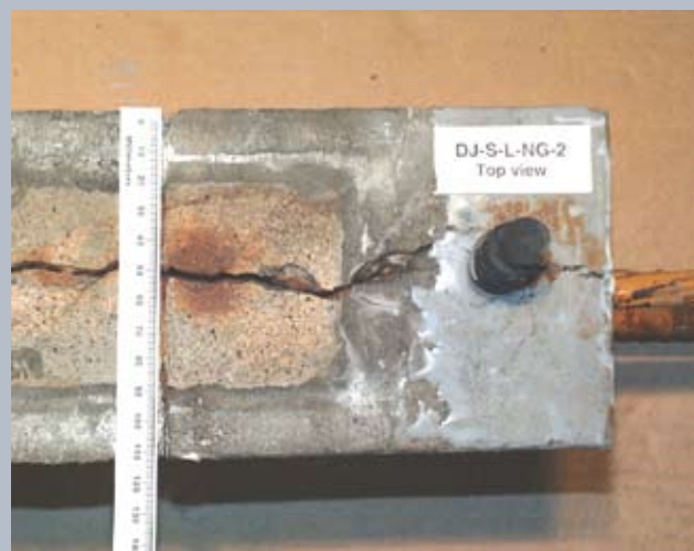
Figure 3. Pictured is an example of specimen condition prior to internal examination for the macrocell corrosion test series. Note: Table 1 defines specimen notations. 1 mm = 0.03937 in.
