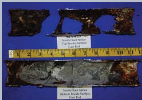
Figure 14. Shown is duct-splice performance from the beam corrosion test series. Note: 1 in. = 25.4 mm.
