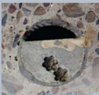
Figure 16. Pictured are bleed-water voids and duct corrosion from the beam corrosion test series.
