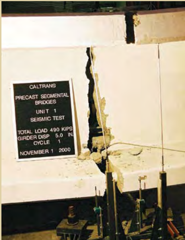
Test unit 100INT explosive tendon failure
