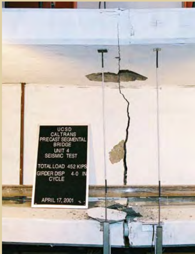
Test unit 50INT/50EXT explosive tendon failure
