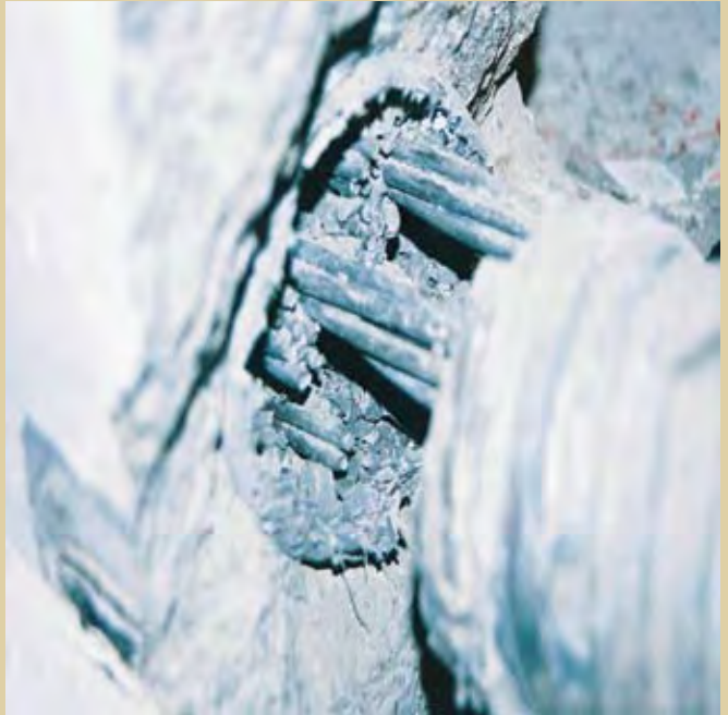
Test unit 100INT explosive tendon failure
