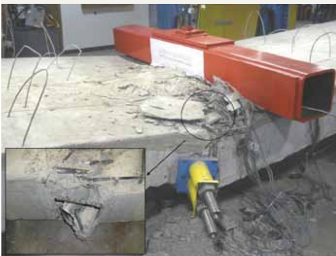
Figure 20. Failure of carbon-fiber-composite cable bridge model.
