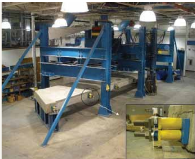
Figure 5. General view of precast, prestressed concrete carbon-fiber-composite cable bridge model.
