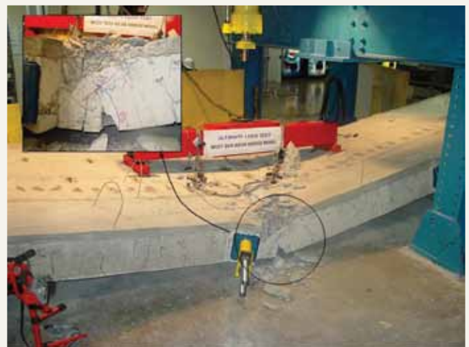
Figure 21. Failure of conventional bridge model.
