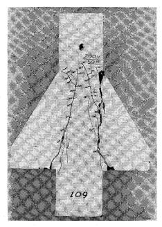
Fig. 21—Shear Failure (S),  $H/V = \frac{1}{2}$
