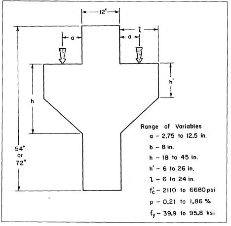
Fig. 5—Corbel Test Specimen
