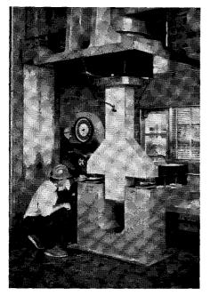
Fig. 9–Test Setup for Vertical Load Only, H/V = 0
