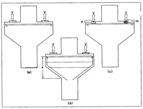
Fig. 6-Reinforcement Details of Test Corbels
