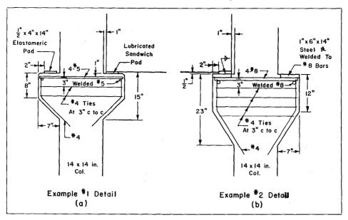
Fig. 4—Corbel Details for Example Problems
