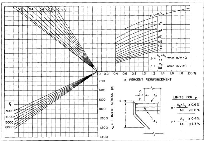
Fig. 3-Design Chart for Ultimate Strength of Corbels
