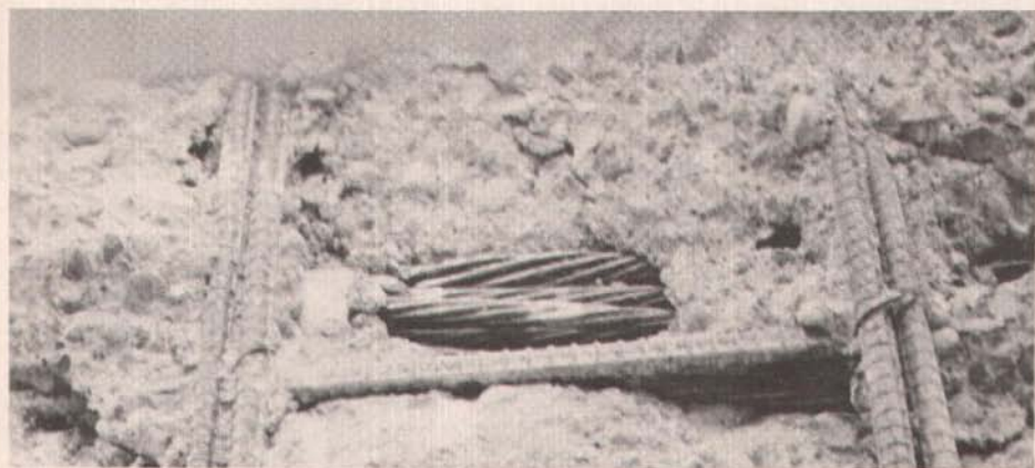
Fig. 10. Slip of dead-end anchor.
