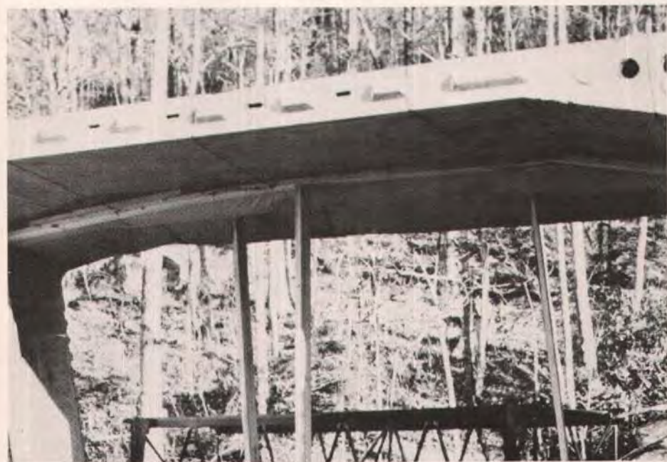
Fig. 4. The test segment being heated with an electric blanket. The blanket was wrapped around the edge of the segment and fastened.
