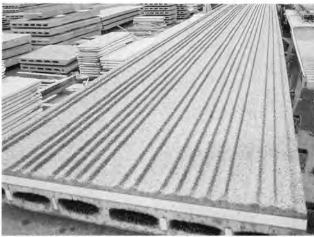
Fig. 10. Exposed aggregate precast wall panel for building in Minneapolis, Minnesota. (Courtesy: Fabcon Incorporated)
