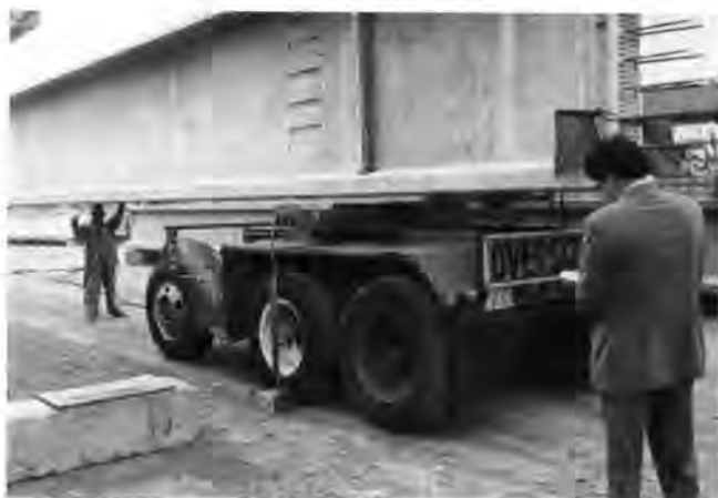
Fig. 19. Measuring roll stiffness of vehicle by placing eccentric loads on vehicle and measuring tilt.
