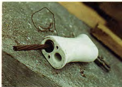
Fig. 12. Center stressing connector used for coupling and tensioning strands.
