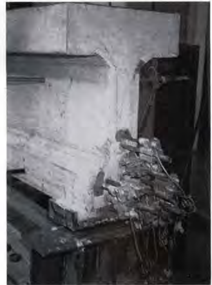
Fig. 5. Electronic potentiometers to measure end slip.
