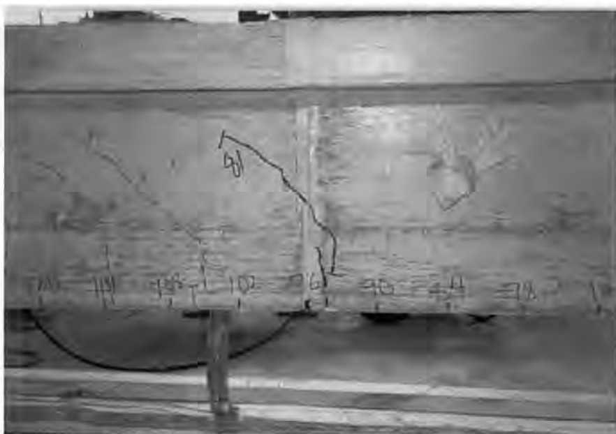
Fig. 20. Test DB850-F2B at load equal to 81 kips (360 kN).
