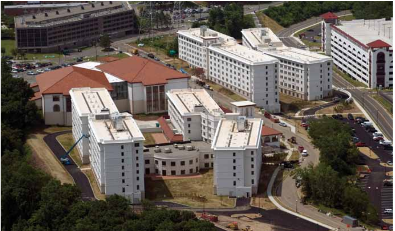
This aerial view shows how the new residence halls at Montclair State University were offset to better align with the topography, reduce the scale of the project and provide a variety of scenic views from the rooms. The foreground halls are located behind the red-roofed recreation center and are connected by the new cafeteria space.
