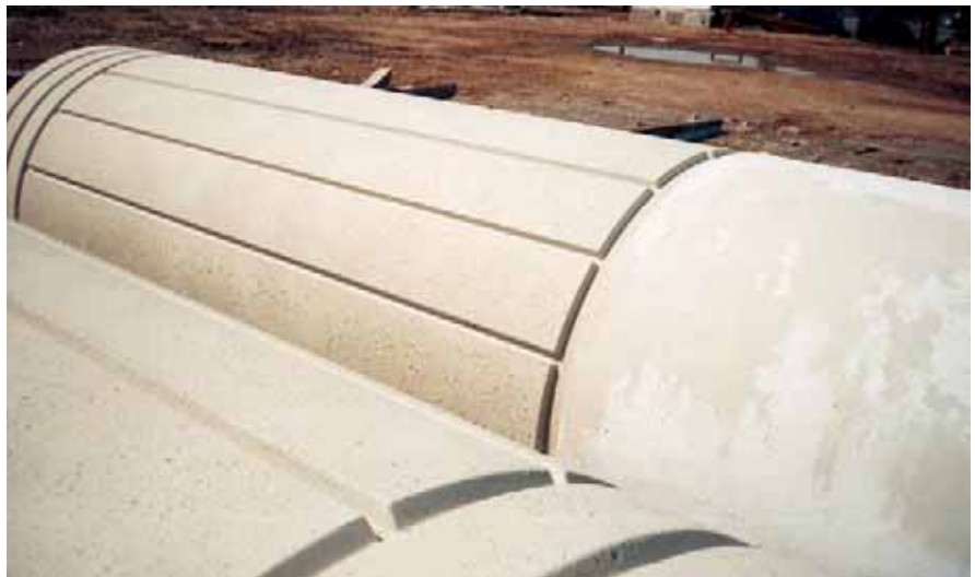
Fig. 9. Column covers in precaster's yard prior to polishing.
