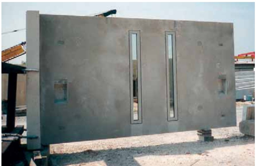
Fig. 10. Panels were cast with 4 in. (102 mm) wide windows and beveled edges, then were completed with a steel window frame and glass that was glazed at the plant. Photo courtesy: Jeffrey Totaro.
